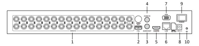
\*: The rear panel of HWD-5216/5224MH-G2 provides 16/24 video input interfaces. HWD-5216MH-G2 provides 2 USB 2.0 interfaces at rear panel, but no USB interface at front panel.
